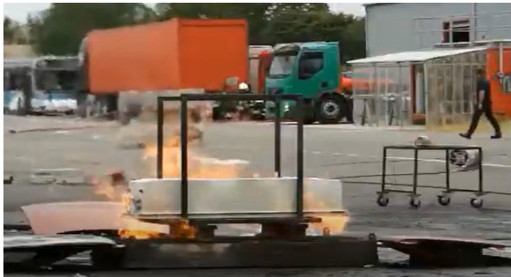
Figure 10. Explosion of the prismatic cells package
