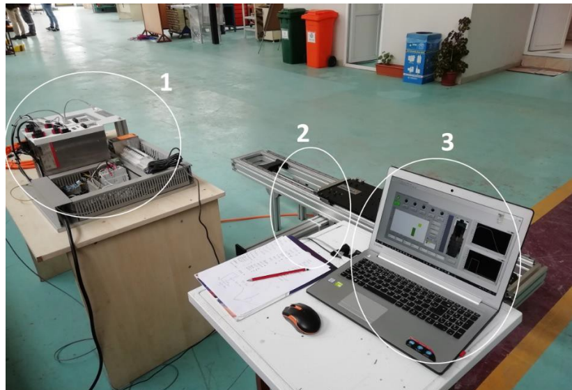
Figure 3. General view of the system implemented, 1. Industrial PC, servo driver, and electrical panel of the system, 2. Servo motor unit, 3. A personal computer where LabVIEW interface is prepared
