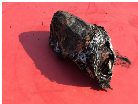
Figure 11. Thermal runaway of cylindrical cells and images after explosion
