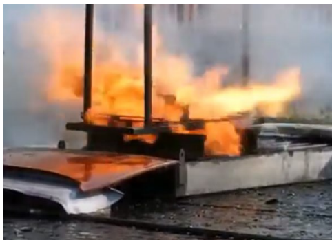
Figure 11. Thermal runaway of cylindrical cells and images after explosion
