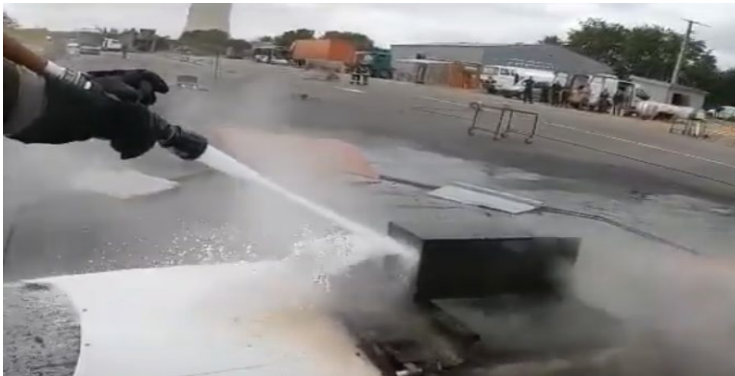
Figure 9. Injection of water through fusible/molten parts
