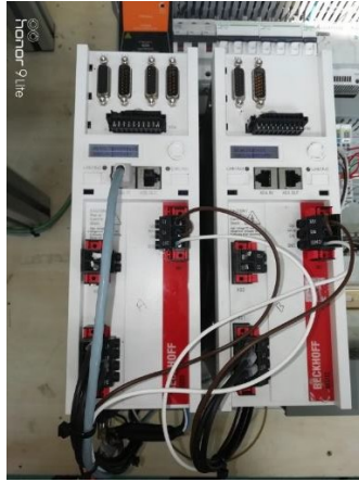
Figure 2. AC servo driver used in the experimental study
